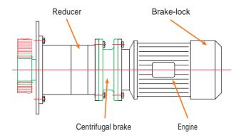
The EC centrifugal brakes consist essentially of a **central core that rotates integrally with the motor shaft**. On its periphery a series of masses are distributed among sectors. These masses are carried by the guides.
